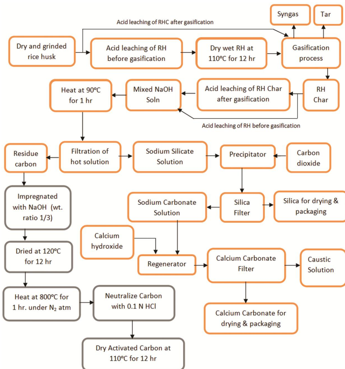
Fig. 2 — Process flow diagram for silica preparation by CO 2 precipitation method.
