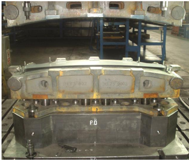
Fig. 7 — Die tools of roof stiffener stamping process.
