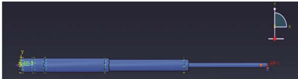
Fig. 3 — CAD model of the considered telescopic cylinder.
