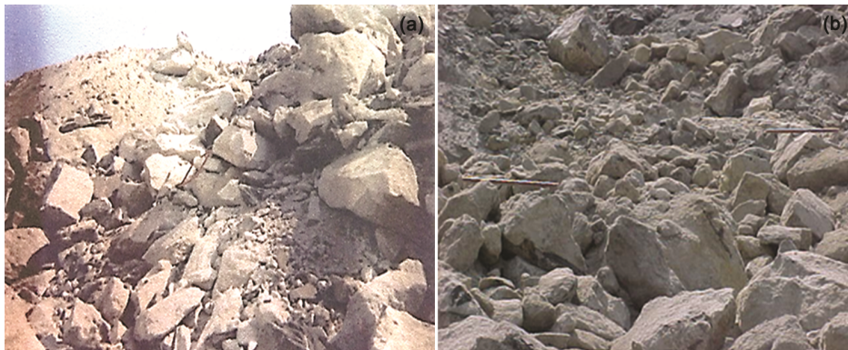
Fig. 3 — (a) Poor fragmentation with large collar boulders and (b) Good fragmentation throughout the muck pile in mine A.
