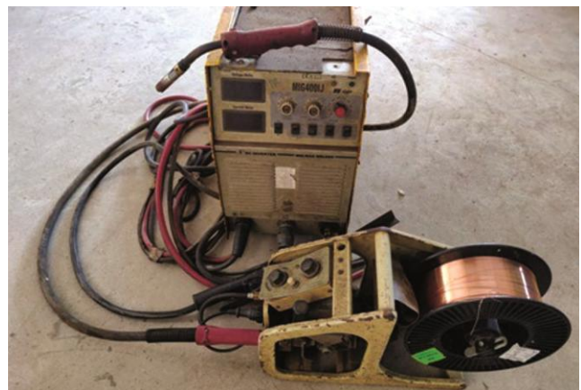
Fig. 1 — Set-up of MIG welding process.
