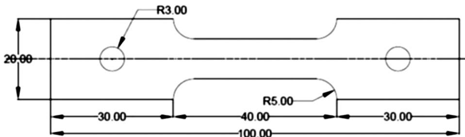
Fig. 3 — Geometry of Fatigue test specimen as per ASTM.
