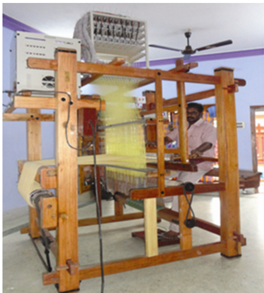
Fig. 3— 128 hooks electronic jacquard loom
