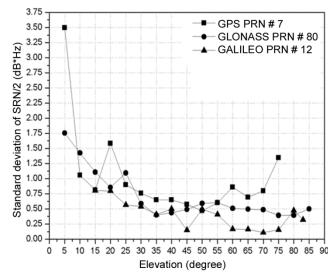
Fig. 5 — Comparison of average signal strength variation on 28 May, 2015
