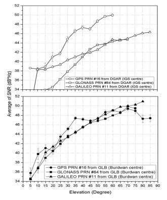
Fig. 8 — Comparison of average and standard deviations of GNSS signal strength for DGAR (top) and GLB, Burdwan for same PRN son 19 June 2018
