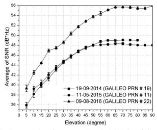
Fig. 4 — Variation of average and standard deviation of signal strengths of E1 C/A signal of different Galileo satellite generations. Galileo PRN #11, PRN#19 (IOV), PRN #22 (FOC)
