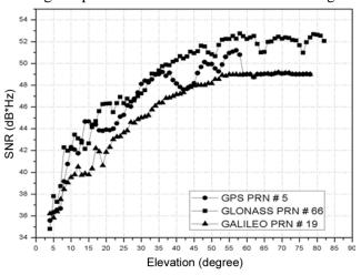
Fig. 1 — Variation of SNR values with increasing elevation angles for GPS, GLONASS and Galileo satellites on 19 September 2014 using JAVAD DELTA G3T receiver
