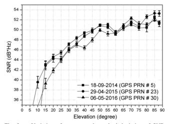
Fig. 2 — Variation of average and standard deviation of SNR values of GPS-L1 signal for different GPS satellite generations. PRN #5 (Block IIR-M), PRN #23 (Block IIR), PRN #30 (Block IIF)
