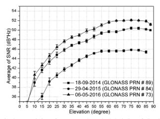
Fig. 3 — Variation of average and standard deviation of signal strength of L1 C/A signal of different GLONASS satellite generations; PRN #89 and PRN #84 (GLONASS M); PRN #73 (GLONASS K)
