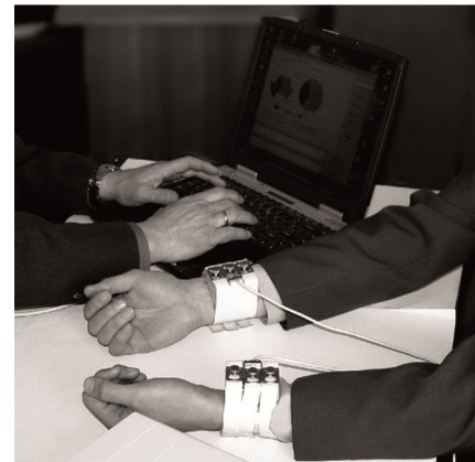
Fig. 2 — Pulse sensors (2 sets of three sensors) for registering sphygmograms (pulsograms) of the radial artery
