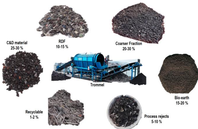
Figure 7: Different bio-mining component at Dhapa landfill
