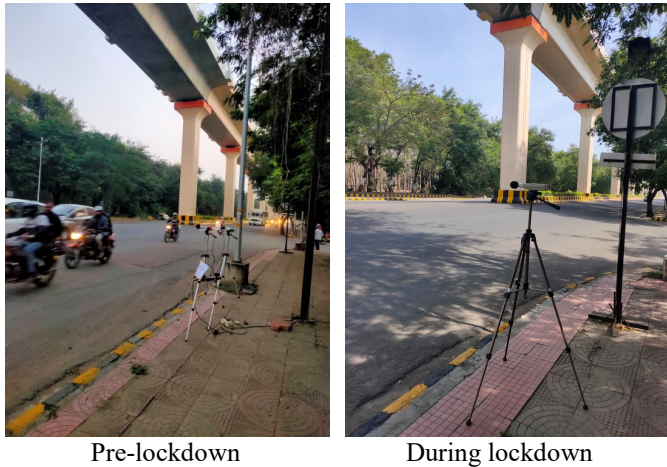
Fig 2: Sound Level Meter Installed at NEERI Gate No. 1 (National Highway) during Lockdown and Pre-lockdown
