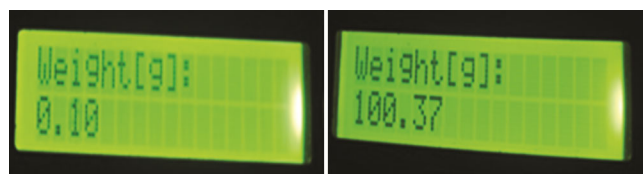
Fig. 4 — Digital weight indicator with LCD at no load and loaded condition
