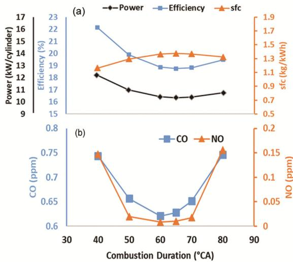
Fig. 11 — Influence of combustion duration on (a) Efficiency, Power and SFC (b) NO and CO
