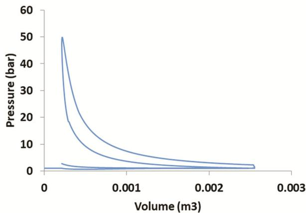
Fig. 5 — P-V diagram for producer gas engine
