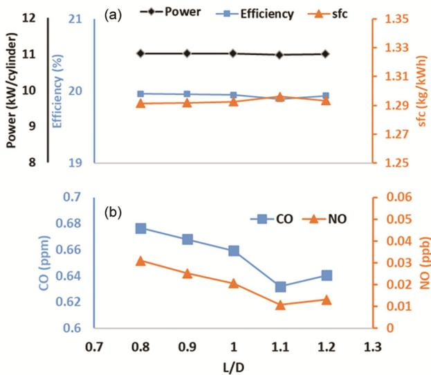
Fig. 9 — Influence of connecting rod length to crank radius ratio (l/r) on (a) Efficiency, Power and SFC; (b) NO and CO
