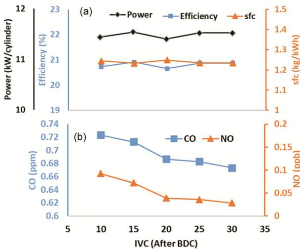
Fig. 12 — Influence of inlet valve closing (IVC) on (a) Efficiency, Power and SFC (b) NO and CO Fig. 12(b)
