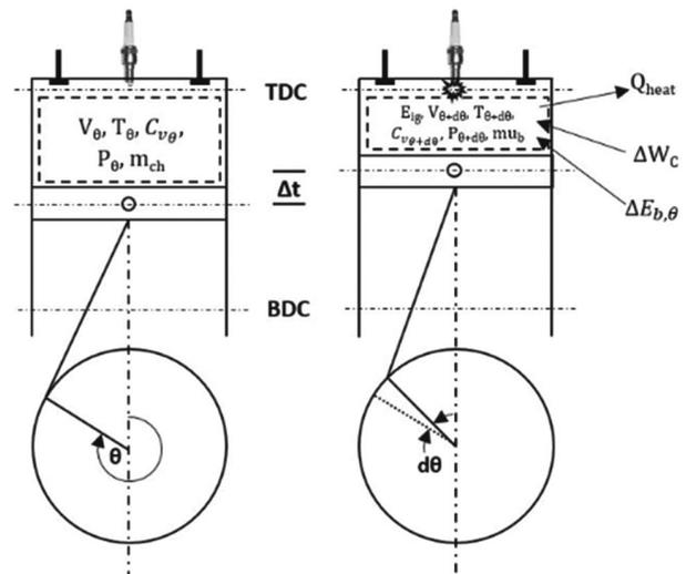
Fig. 1 — Control volume of combustion process during compression stroke before and after 'dθ' interval of crank angle
