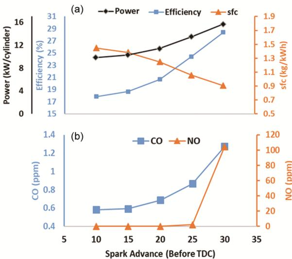
Fig. 10 — Influence of spark advance on (a) Efficiency, Power and SFC; (b) NO and CO
