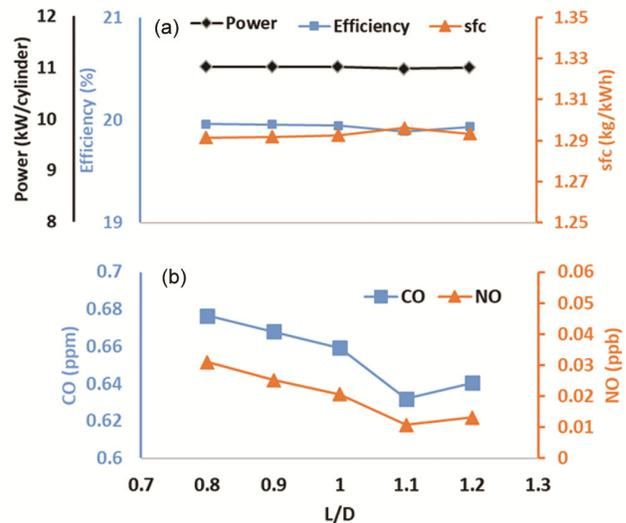
Fig. 8 — Influence of stroke to bore (L/D)ratio on (a) Efficiency, power and SFC; (b) NO and CO
