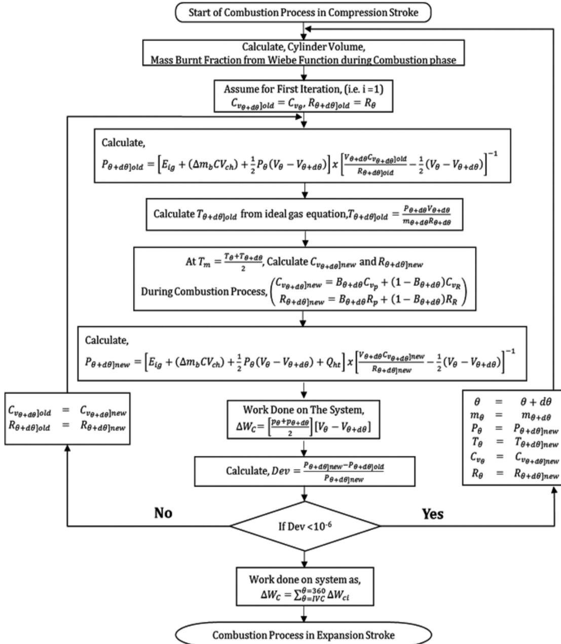
Fig. 2 — Solution procedure of combustion process till the completion of compression stroke
