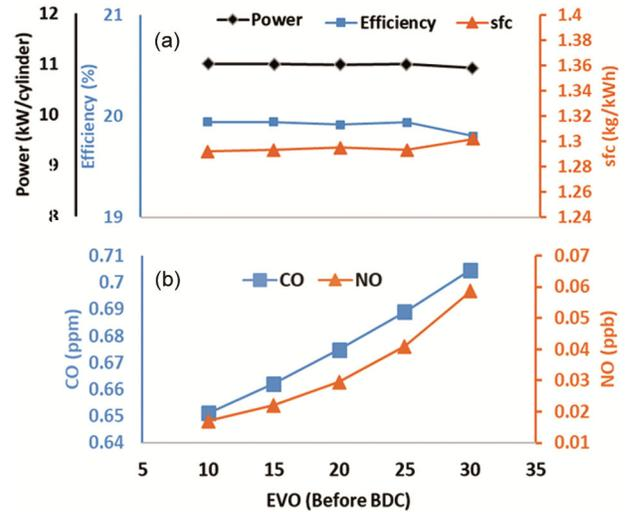
Fig. 13 — Influence of exhaust valve opening (EVO) on (a) Efficiency, Power and SFC; (b) NO and CO Fig. 11(b)
