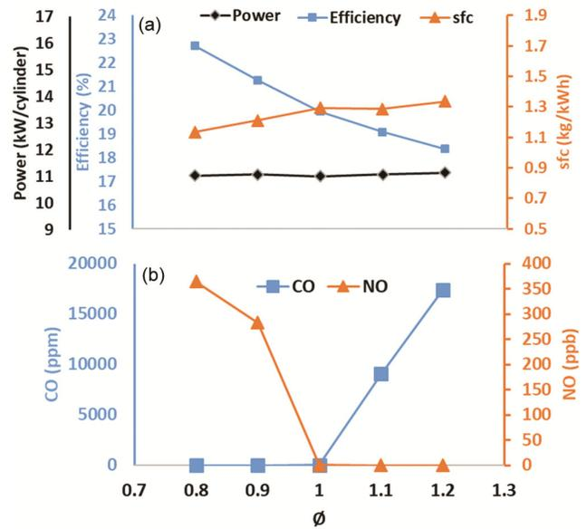
Fig. 7 — Influence of fuel-air ratio ( $\phi$ ) on (a) Efficiency, Power and SFC; (b) NO and CO emission
